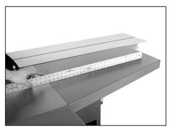
Figure 21. Checking with a straightedge.
